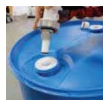
Vent port on the coupler may either be left open to vent to atmosphere or be outfitted with a check valve to allow make-up air into the drum.
