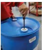
A large flat blade or #4 Phillips screwdriver may be used to remove shipping plug.
