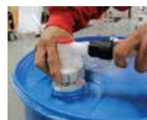
Turn Coupler Lock Ring clockwise fully until stop is reached to connect and open.
